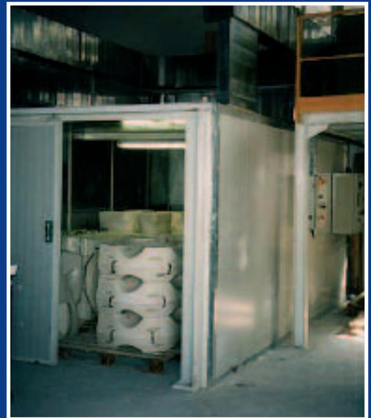
Intermittent dryer type ES 5 for plaster moulds
