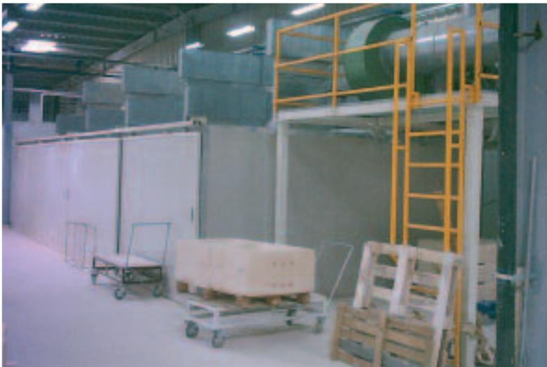
Intermittent dryer type ES 10 for plaster moulds
