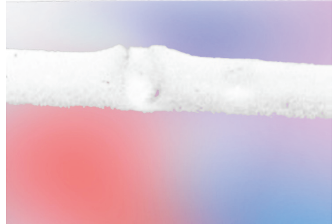
Fig. 2: Case 2 Cross-section of a pinhole.
